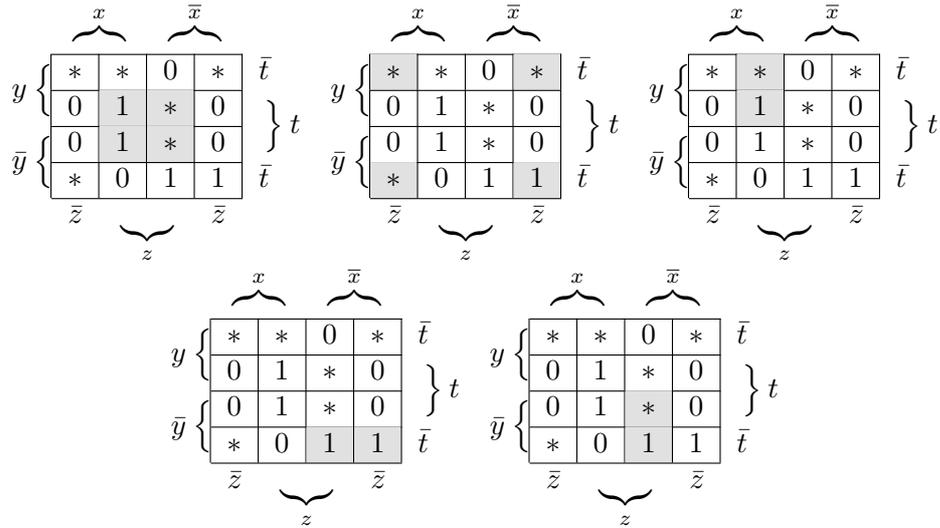
Soit  $\mathcal{M}(f) = \{zt, \bar{z}\bar{t}, xyz, \bar{x}\bar{y}\bar{t}, \bar{x}\bar{y}z\}$ .
